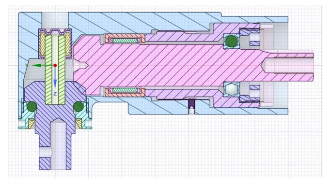
Assemble the seal and retainer that is not shown.
